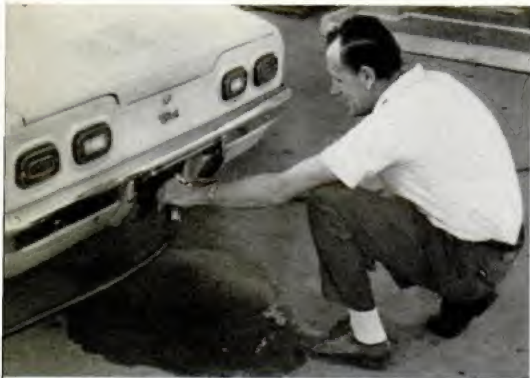
VEGA FILLER NECK is inconvenient to use and the filler pipe angle allows spillage when topping off
